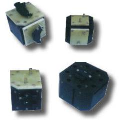
Most Cube fixtures under 6.0" are made from billet tooling plate. These Cubes shown range from 3.0" to 5.0" and are for testing automotive ignition components.
